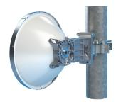
0.3 m | 1 ft ValuLine® High Performance Low Profile Antenna, single-polarized, 37.000 – 40.000 GHz, OEM custom flange, white antenna, gray radome without flash, standard pack—one-piece reflector
