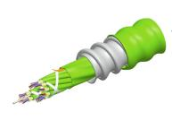
Fiber indoor cable, Plenum MPO Trunk, interlocking aluminum armored with plenum jacket, 128 fiber multi-unit with 16 fiber subunits, Gel-free, OM5 multi-mode, Feet jacket marking, Lime green jacket color
