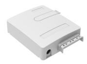
Wall-mountable Optic fiber outlet with one LC/APC shuttered Duplex adapter and no pigtails, for ANT splice protection
