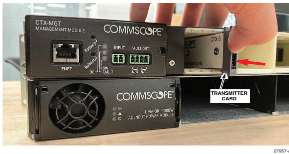
Figure 9. Inserting a Transmitter Card
