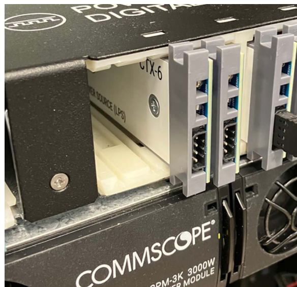
Figure 10. Fully Inserted Transmitter Card
