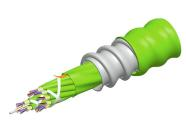
Fiber indoor cable, LazrSPEED® Plenum MPO Trunk, interlocking aluminum armored with plenum jacket, Multimode OM5, 24 fiber multiunit with 8 fiber subunits, Lime-green jacket color, Feet cable marking
