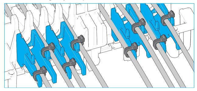
1 Guide the cables in the external drop cable guidance bracket and attach with a cable tie as shown.
