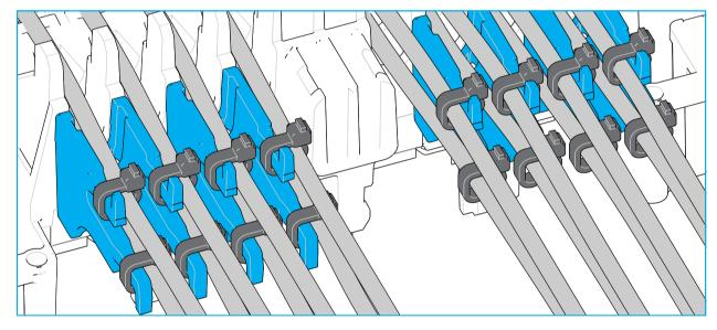
1 Guide the cables in the external drop cable guidance bracket and attach with a cable tie as shown.
