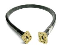
FlexTwist® Flexible Twist for WR229, 3.54–4.2 GHz, with interface types UDR40 and UDR40, 900 mm
