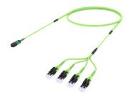
Ultra Low Loss ULL OM5 MPO8 APC non-pinned to LC/UPC Uniboot Ruggedized fanout Cable, 8-Fiber, Dual Rated (OFNR/LSZH), 8 fiber PmP 2.0 mm
