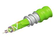
Fiber indoor cable, LazrSPEED® Plenum MPO Trunk, interlocking aluminum armored with plenum jacket, Multimode OM5, 96 fiber multiunit with 12 fiber subunits, Lime-green jacket color, Feet cable marking
