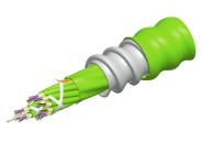
Fiber indoor cable, LazrSPEED® Plenum MPO Trunk, interlocking aluminum armored with plenum jacket, Multimode OM5, 288 fiber multiunit with 12 fiber subunits, gel-free, Feet jacket marking, Lime-green jacket color
