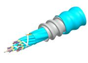
Fiber indoor cable, LazrSPEED® Low Smoke Zero Halogen Riser MPO Trunk, interlocking aluminum armored with low smoke zero halogen riser jacket, Multimode OM4, 24 fiber, Gel-free, Feet jacket marking, Aqua jacket color, B2ca flame rating
