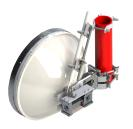
0.6 m | 2 ft ValuLine® High Performance Low Profile Antenna, dual band, dual polarised 71.000 – 86.000 GHz and dual polarised 17.700 - 19.700 GHz, OEM custom flange
