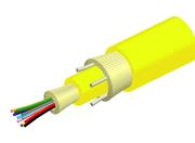
Fiber indoor cable, Low Smoke Zero Halogen Riser MPO Trunk, with 2.0 mm Subunits, 12 fiber, Singlemode G.657.A2/B2, Gel-free, Feet jacket marking, Yellow jacket color, B2ca Flame rating
