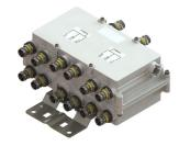
Compact Quad Triplexer 612-960/1695-2700/3300- 4200 MHz, 4.3-10 connectors, DC sense
