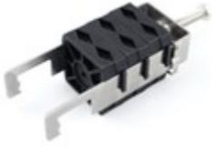
KwikClamp™ Hanger for power & fiber cables, one 7-9 mm hole and one 22-34 mm hole (alongside each other), quadruple block; includes hardware
