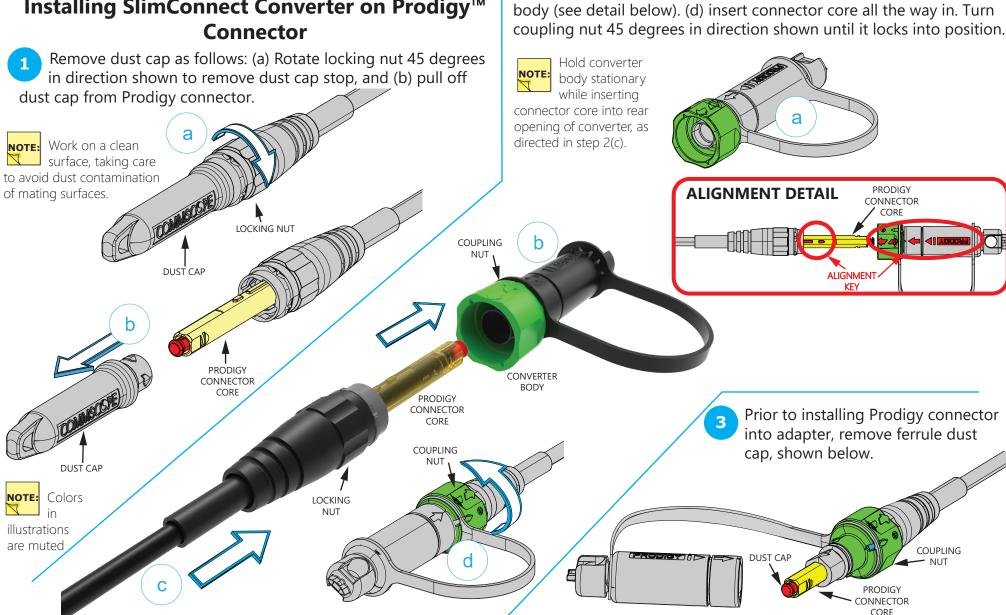
Install the converter as follows: (a) Locate Prodigy SlimConnect converter, (b) hold onto converter body, (c) align alignment key
