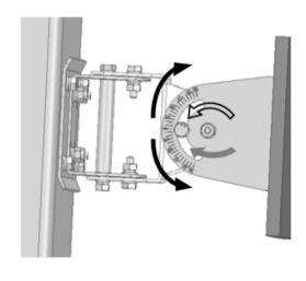
1. Loosen the three fixing screws at the left- and right-hand side. (Do not unscrew them completely.)
