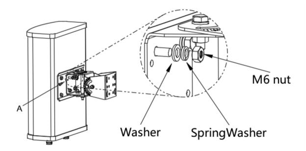
Attach antenna and fasten with washers and M6 nuts (M6 torque: 10 Nm).
