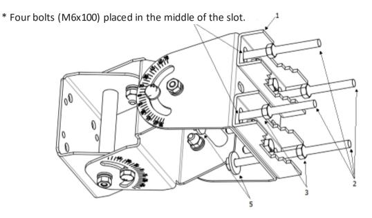
Insert four M6x100(2) bolts and four filled-corner washers (5) into the antenna mounting bracket; then, tighten the four M6 nuts (3), four M6x100 (2) placed in the middle of the slot.
