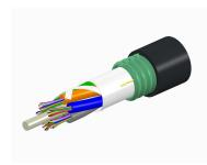
Fiber OSP cable, LightScope ZWP® Single Jacket/Single Armor, 288 fiber, Gel-Free, Stranded Loose Tube, Singlemode G.652.D and G.657.Al, Feet jacket marking, Black jacket color
