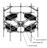
PIM Optimized Adjustable 4-Sector Monopole Platform with 13ft Face - 2-7/8in OD Face Pipes & Top Rail - Includes (12) 2-7/8in OD x 120in Antenna Pipes
