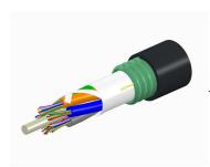
Fiber OSP cable, TeraSPEED® Single Jacket/Single Armor, 144 fiber, Gel-Free, Stranded Loose Tube, Singlemode G.652.D and G.657.A1, Feet jacket marking, Black jacket color
