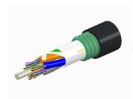
Fiber OSP cable, LazrSPEED® Single Jacket/Single Armor, Gel-Free, Stranded Loose Tube, 24 fibers, Multimode OM3, Feet jacket marking, Black jacket color
