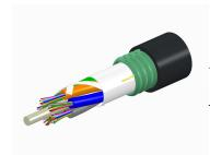
Fiber OSP cable, LazrSPEED® Single Jacket/Single Armor, Gel-Free, 36 fibers, Stranded Loose Tube, Multimode OM3, Feet jacket marking, Black jacket color
