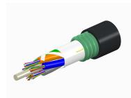
Fiber OSP cable, LazrSPEED® Single Jacket/Single Armor, , 60 fibersGel-Free, Stranded Loose Tube, Multimode OM3, Feet jacket marking, Black jacket color
