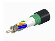
Fiber OSP cable, LazrSPEED® Single Jacket/Single Armor, 144 fiber, Gel-Free, Stranded Loose Tube, Multimode OM3, Feet jacket marking, Black jacket color
