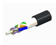
Fiber OSP cable, TeraSPEED® Single Jacket All-Dielectric, 60 fibers, Gel-Free, Stranded Loose Tube, Singlemode G.652.D and G.657.Al, Feet jacket marking, Black jacket color
