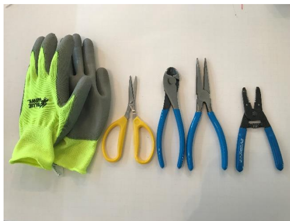
Figure 1: Cable preparation tools used include gloves, scissors, side cutters, needle nose pliers, and wire strippers
